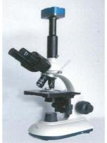
E 5 T Trinocular Microscope with Achromat Objectives: Trinocular Head inclined at 30 deg Beam splitter 50/50: Eyepieces WF10x(18): Achromat or Plan Achromat Objectives A4x, A10x, A40x, A100x(oil): Nosepiece reversed 4 positions: Co-Axial course and fine focusing knobs: Co-Axial Mechanical Stage with specimen holder Condenser Abbe 1.25 with iris diaphragm with rack & pinion adjustment: Illumination variable LED with Lithium battery (approx 8hrs) Blue filter, built in with. All prices include GST.
